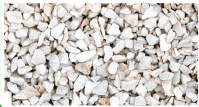
CLEANING EXCAVATION AND CREATION OF A GRAVEL DRAINING BED 5-20 MM
